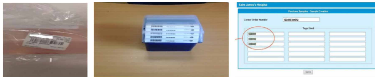
Figure 2: The RFID-enabled tracking system and RFID tags on sample bags
