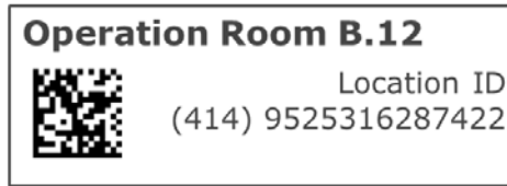
Figure 4-1 Application Identifier (414) – GLN of a physical location
