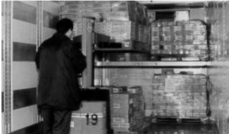
Figure 28: Double deck trailer and/or beam trailer (T&B)
