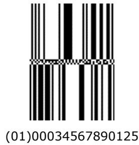
Abbildung 5.5.2.1.4-1. GS1 DataBar Stacked Omnidirectional
